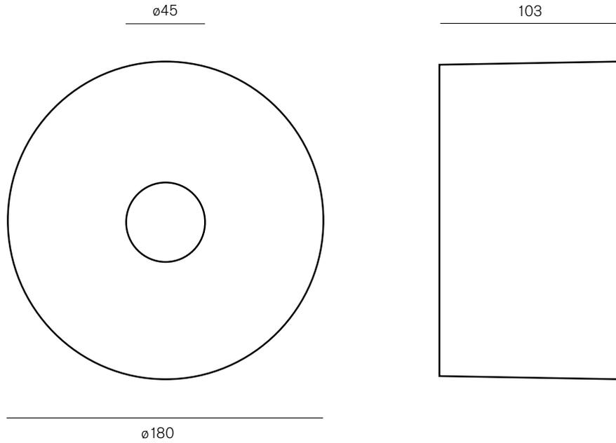
Material: Cast Aluminium or Cast Gunmetal
