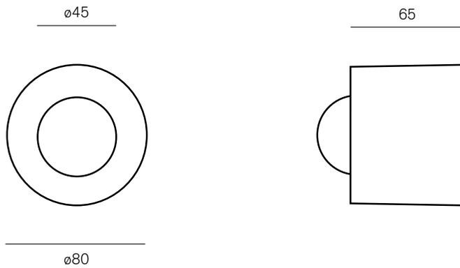
Material: Cast Aluminium or Cast Gunmetal
