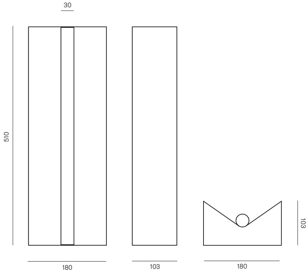
Material: Cast Aluminium or Cast Gunmetal
