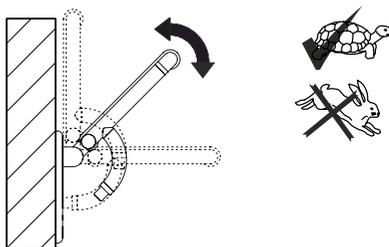
Check friction on both sides of the seat.
