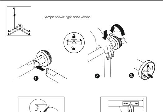
When joining the rails, note the sticker and hold the rails at right-angles to each other.
