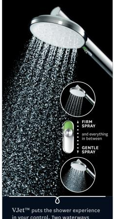
in your control. Two waterways converge in a chamber behind each nozzle to create a spinning vortex that seamlessly changes speed as you adjust the slider. Resulting in a smooth transition from a firm invigorating spray, to a gentle spray, and everything in between - uniquely tailored by you.
