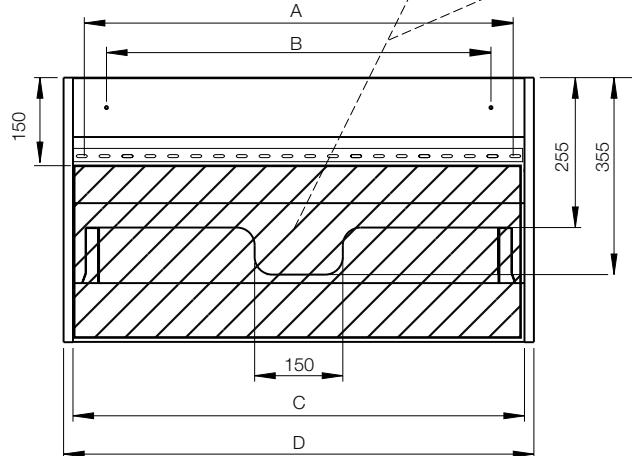
\* Recommended positions for under cabinets with integrated wash basin
