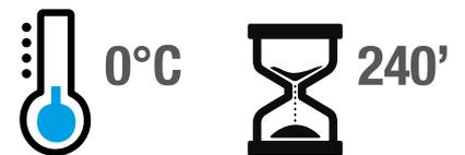
Concrete setting time is function of the air temperature. A rough indication is 60' at 30°C, 120' at 18°C. 240' at 0°C. Please follow the prescriptions of concrete supplier.
