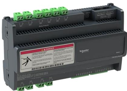
Installed with SpaceLogic (formerly known as SmartX) RP-C controllers, it provides high-performance relays with high inrush current capability, and is well suited for LED lighting applications. Its 10 relay outputs are ideal for controlling lights and blinds in less complex installations.
