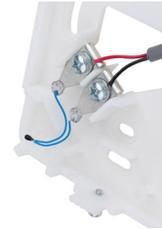
5. With sensor base fully installed, align top of cover to mounting tabs on top of sensor base. Swing cover downward until it latches at the bottom.
