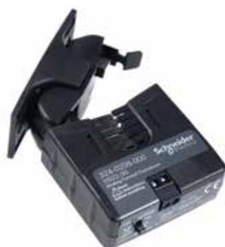
The Schneider Electric range of current transducers delivers high performance, reliable current monitoring for applications including fan status, belt loss, and most Variable Speed Drive (VSD) applications. Current transducers detect changes in a conductor's current/ampereage and provide an analog output to Building Management System (BMS) controllers. The current transducers are available in solid-core versions for new projects and split-core versions to accommodate retrofits.
