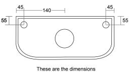
from the underside of the tank (ie plumbing pipe position)
