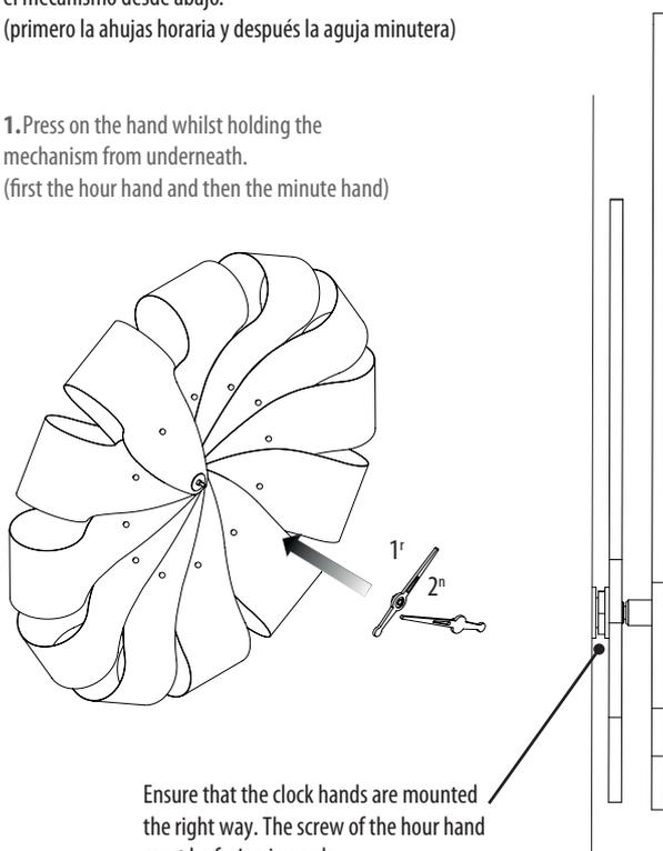
Ensure that the clock hands are mounted the right way. The screw of the hour hand must be facing inwards.
