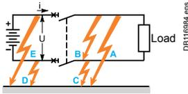
DE116984.eps | <b>- (or +) earthed</b><br>+ and - conductors protected and disconnected<br>
