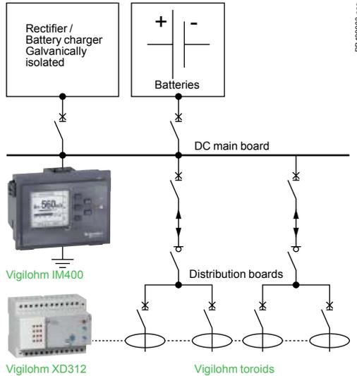
The Insulation Fault Locator detects the injected current from the IM400 through its toroid. The IM400 injects a low frequency component on the network (2.5 Hz) which allows measuring the network insulation, and locating the insulation fault. XD312 type of locator is suited for the automatic location of low impedance faults (typically less than 1 kOhm).
