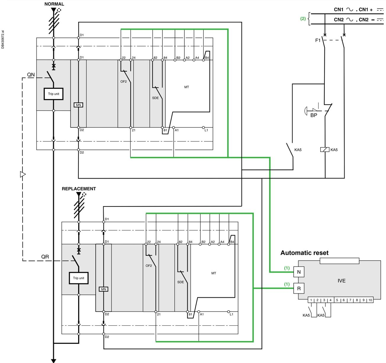
[1] Prefabricated wiring supplied.
