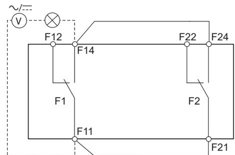
**NOTE:** terminal capacity for auxiliary contact is AC250 V 2 A.
