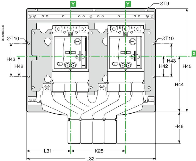
**Note:** coupling accessory: only for changeover systems using fixed versions of ComPacT NSX circuit breakers.
