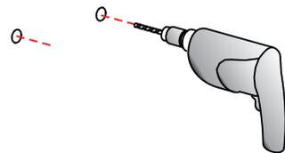
Using a 6mm drill bit, drill holes on the marked positions.
