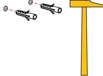
Insert the rawl plugs into the drilled holes.
