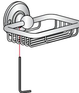
Insert the Soap Basket body into the base. Fix it with the allen key supplied.
