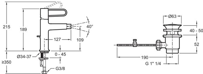
Product Specification: Customizable single-lever bidet mixer, with waste. E21033-BL. Collection: ODÉON RIVE GAUCHE. DIMENSIONS: 18.30 x 4.50 cm. WEIGHT: 1.3 kg. MATERIAL: Brass. INSTALLATION TYPE: 1 hole. TYPE: Single-lever. FLOW RATE: 5 l/mn. HEIGHT UNDER SPOUT: 189. SPOUT PROJECTION: 127. CONNECTION: With supply hoses. WASTE : Yes.
